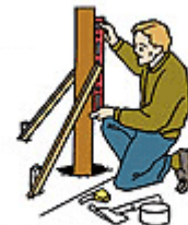
Use a level to make sure each post is in an exact, upright position.
