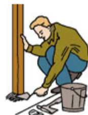
Build a mound around each post to eliminate standing water.
